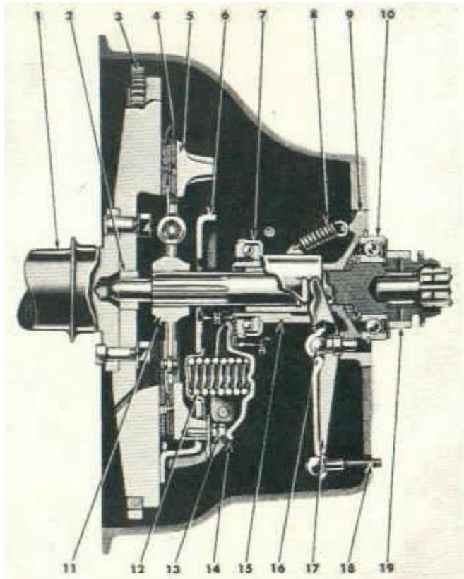
**FIG. 21 CLUTCH ASSEMBLY**
