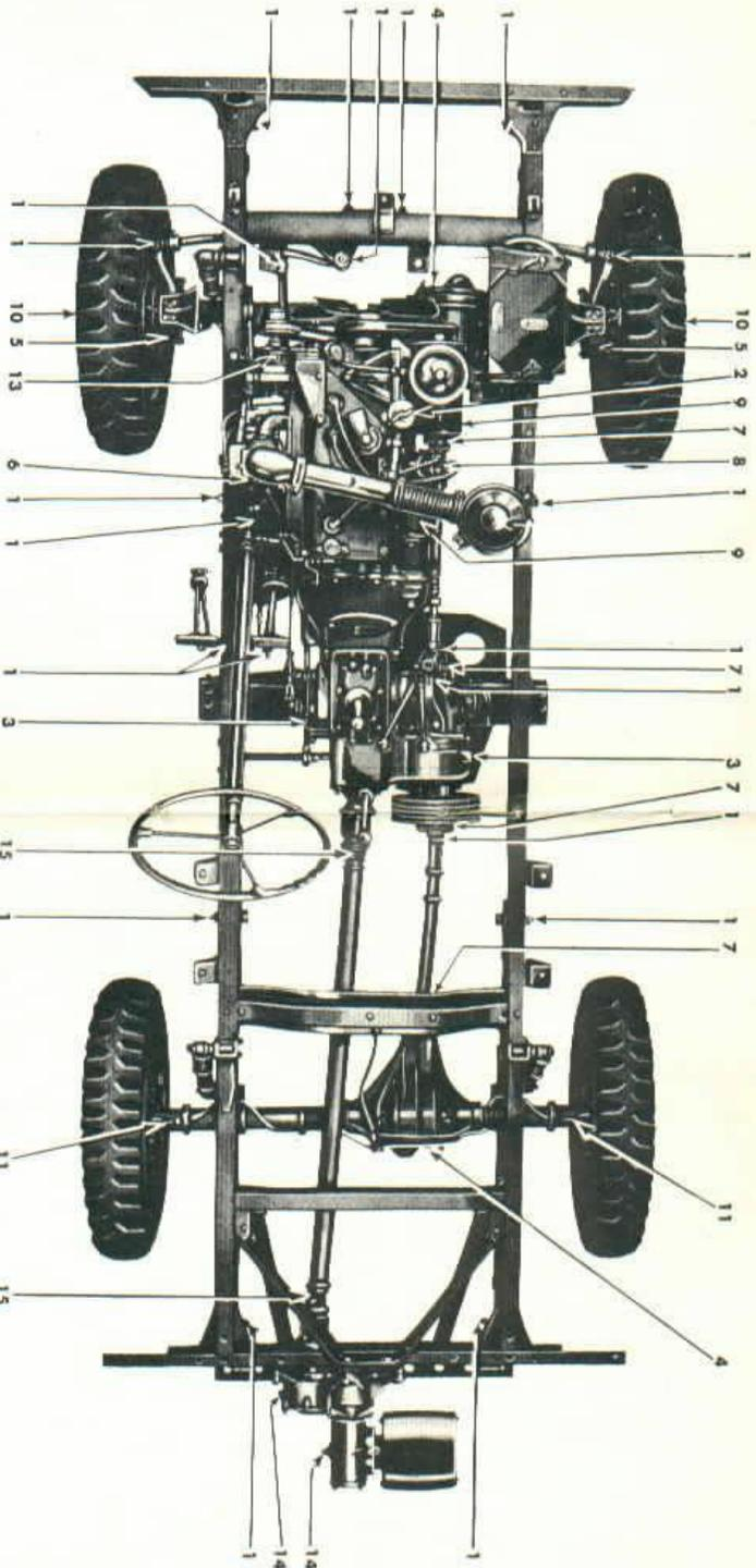
FIG. 20—CHASSIS, SHOWING PARTS REQUIRING LUBRICATION
