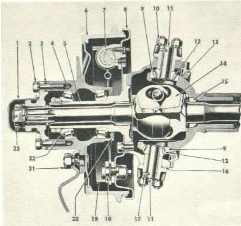
FIG. 25 FRONT STEERING KNUCKLE
