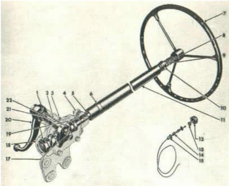
FIG. 31--STEERING GEAR
