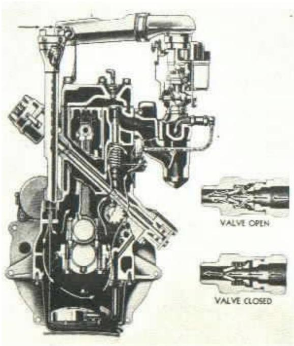
FIG. 12—CRANKCASE VENTILATING SYSTEM
