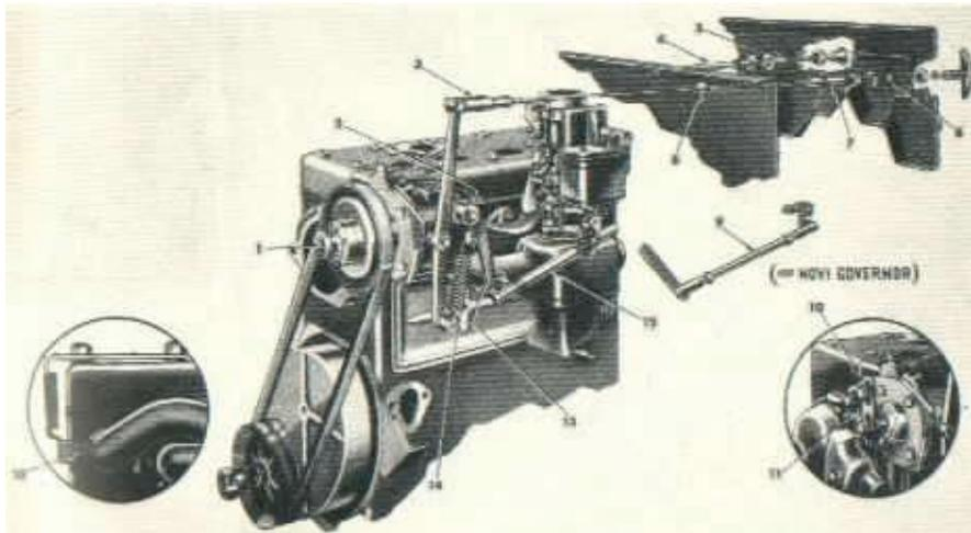
FIG. 34—GOVERNOR INSTALLATION AND ADJUSTMENT
